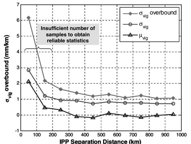
Fig. 4  $\sigma_{vig}$  overbound results from the station-pair method and WAAS supertruth data for a quiet day (2 July 2000).
