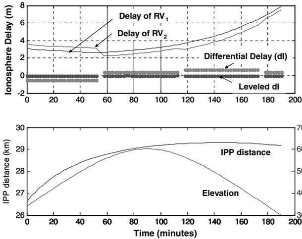
Fig. 7 Bias-removed differential ionosphere slant delays from JPL postprocessed CORS data.
