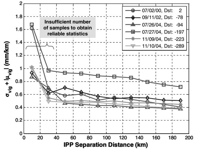
Fig. 9  $\sigma_{vig} + |\mu_{vig}|$  results from the station-pair method and JPL-CORS data for all six days (with noise reduction and bias removal).
