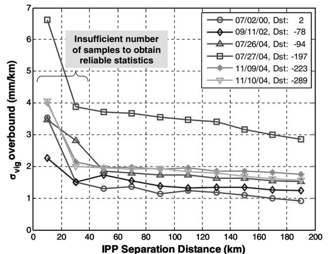
Fig. 10  $\sigma_{vig}$  overbound results from the station-pair method and JPL-CORS data for all six days (with noise reduction and bias removal).
