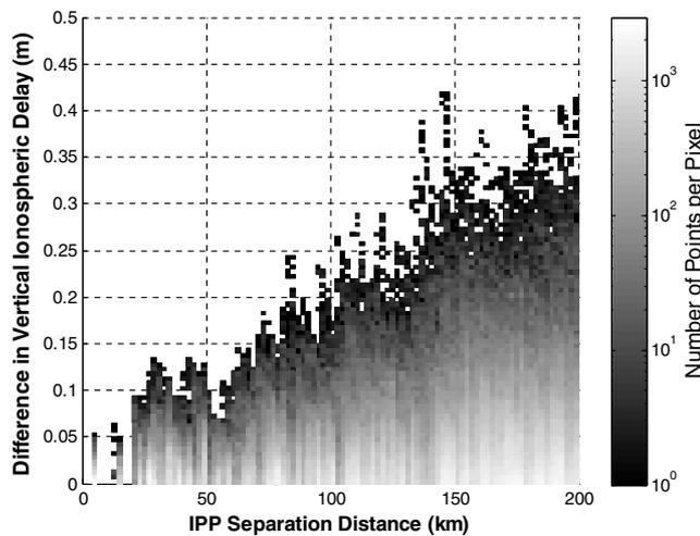
Fig. 8 Differential vertical ionosphere delay results on a quiet day (2 July 2000) from the station-pair method and JPL-CORS data (with noise reduction and bias removal).
