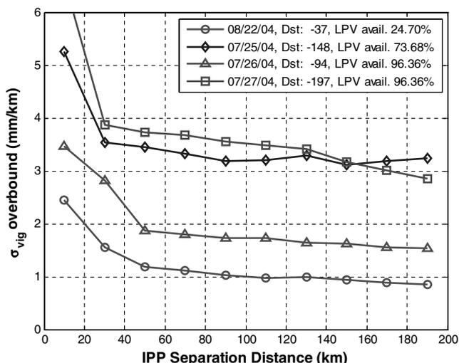
Fig. 12  $\sigma_{\text{vig}}$  overbound results of WAAS-affected days from the station-pair method and JPL-CORS data.
