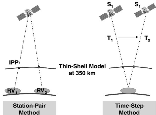
Fig. 1 Satellite and receiver configuration for the station-pair and time-step methods.
