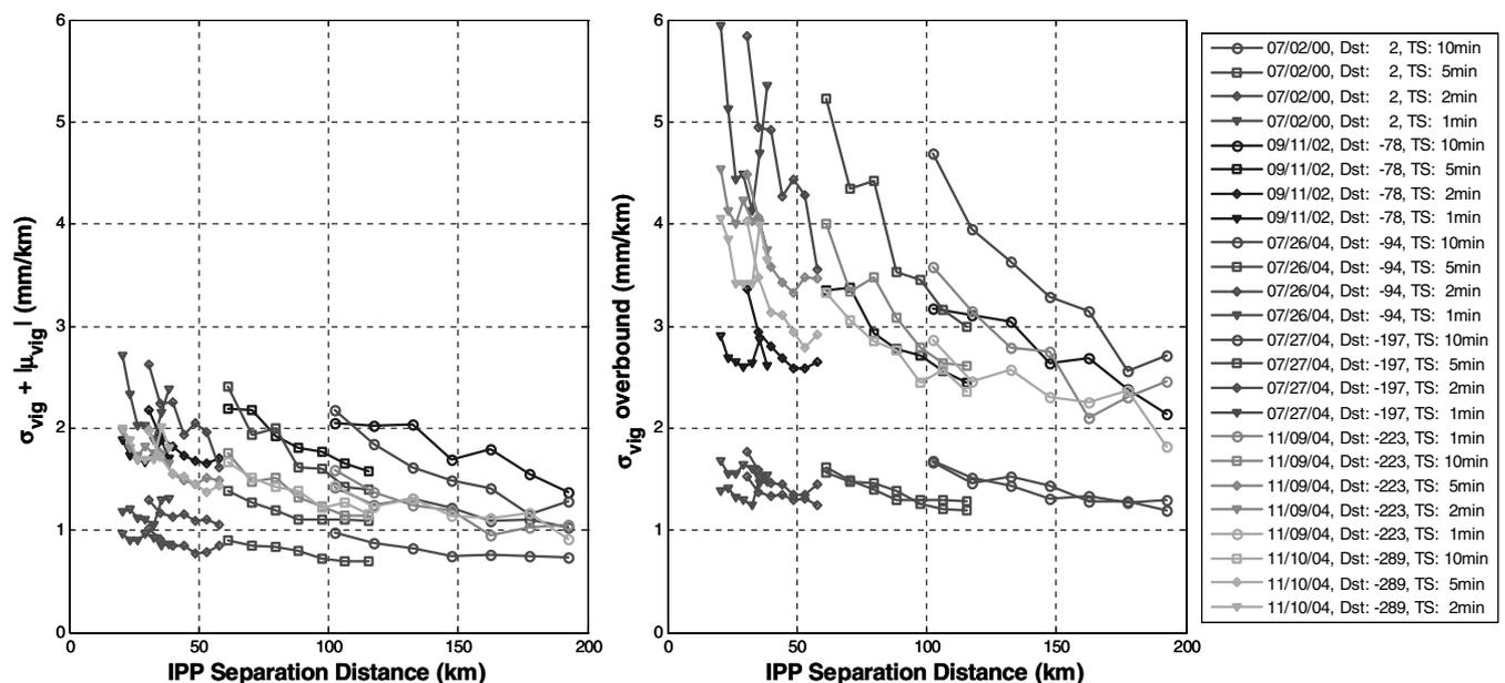
Fig. 6  $\sigma_{\text{vig}}$  overbound results from the time-step method and WAAS supertruth data for all six days.
