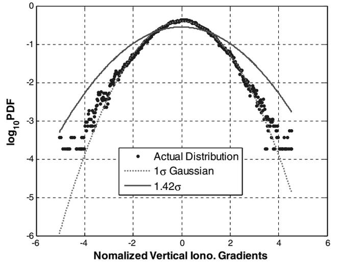
Fig. 3 Probability density function of normalized vertical ionospheric gradients on a quiet day (2 July 2000).
