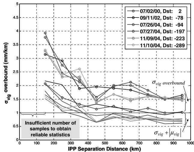
Fig. 5  $\sigma_{\text{vig}}$  overbound results from the station-pair method and WAAS supertruth data for all six days.
