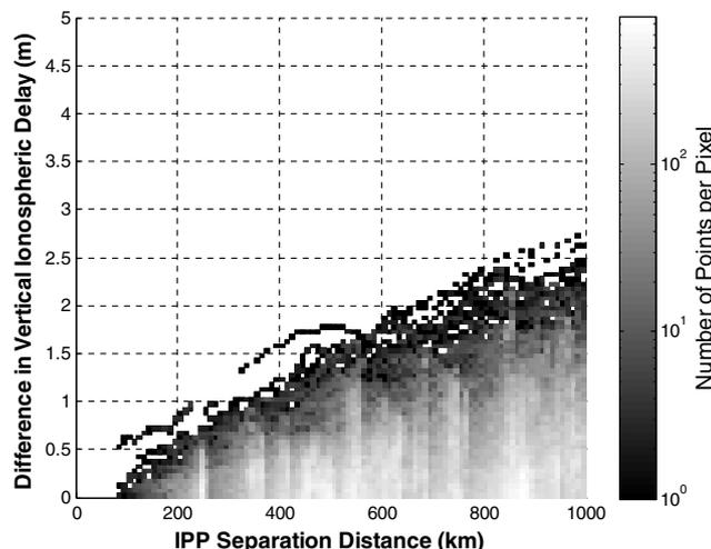
Fig. 2 Differential vertical ionospheric delay results on a quiet day (2 July 2000) from the station-pair method and WAAS supertruth data.
