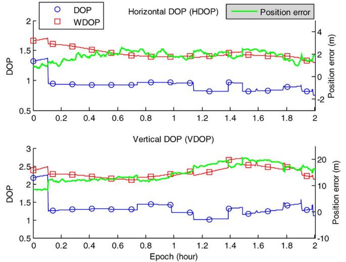
Fig. 4. Comparison of the DOP, WDOP, and position error in the horizontal and vertical directions over 2 h.
