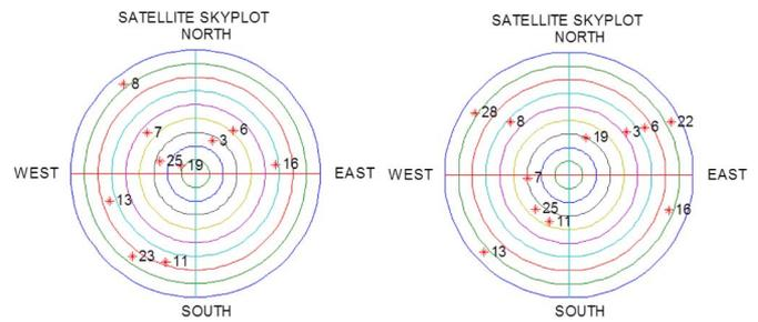
Fig. 6. Visible satellite distribution (left: 0.2 h; right: 1.3 h).
