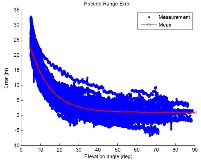
Fig. 3. Pseudorange error with respect to elevation angles.
