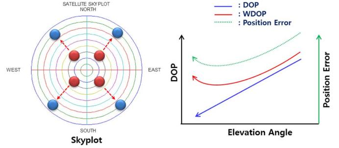
Fig. 1. (Right) DOP, WDOP, and position error changes according to (left) satellite elevation angle changes.
