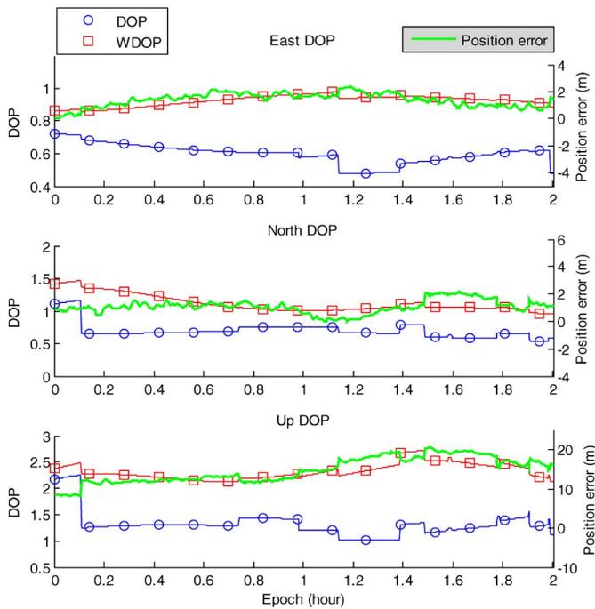
Fig. 5. Comparison of the DOP, WDOP, and position error in the East–North–Up directions over 2 h.
